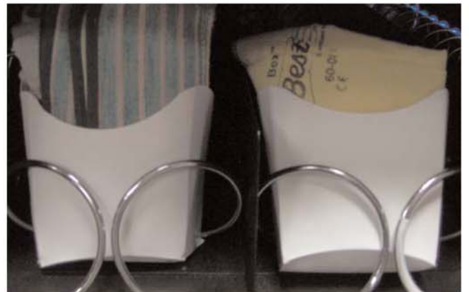
leather welding gloves and kevlar gloves stored and dispensed in french fry containers to ensure proper vending
